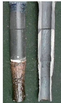
Fig.12 Ladle shroud performance at Caster A and the cut section after use.
